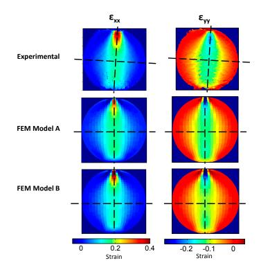
**Figure 8.** Strain maps in X direction (considered normal to indentation) and Y direction (considered in the direction of the indentation) Obtained experimentally (upper row), and numerically with FEM A and B (central and lower rows).
