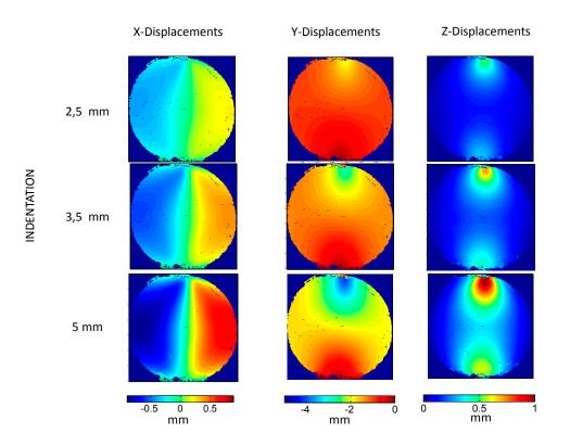
**Figure 7.** Displacement maps obtained experimentally at 2.5 mm (first row), 3.5 mm (second row) and 5 mm (third row) indentation obtained in Xcdirection (first column), Y direction (second column), and Z direction (third column).
