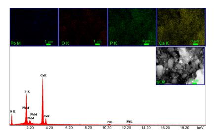
Figure 12. EDX spectrum and elemental mapping of CD-HAp\_1 sample after the adsorption of Pb<sup>2+</sup>.
