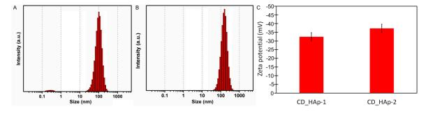
**Figure 1.** Particle size distribution measured by DLS of: CD-HAp\_1 (**A**); and CD-HAp\_2 (**B**) nanoparticles suspensions. Zeta potential of CD-HAp\_1 and CD-HAp\_2 nanoparticles suspensions (**C**).
