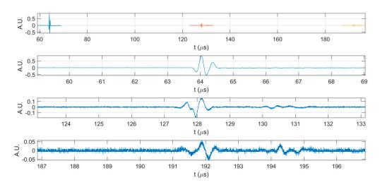
Figure 3. The first three echoes acquired for CD-HAp\_1 sample: together (top); and separated (below).
