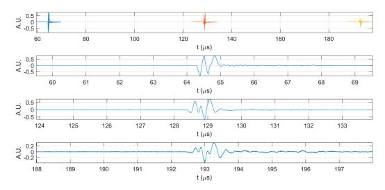
Figure 2. The first three echoes acquired for double-distilled water: together (top); and separated (below).
