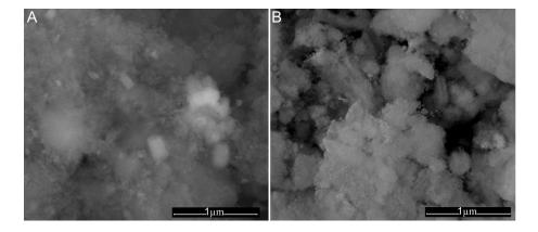
Figure 11. SEM images of: CD-HAp\_1 (A); and CD-HAp\_2 (B) samples after the adsorption of Pb<sup>2+</sup>.
