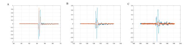
**Figure 4.** Detailed comparison between the first three echoes registered for double-distilled water (blue) and CD-HAp\_1 solution (orange). First echo (**A**), second echo (**B**) and third echo (**C**).
