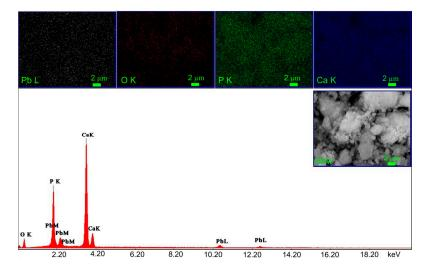
Figure 13. EDX spectrum and elemental mapping of CD-HAp\_2 sample after the adsorption of Pb<sup>2+</sup>.
