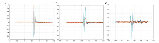
**Figure 6.** Detailed comparison between the first three echoes registered for double-distilled water (blue) and CD-HAp\_2 solution (orange). First echo (**A**), second echo (**B**) and third echo (**C**).
