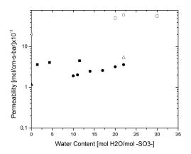
**Figure 6.** Hydrogen permeability. Schalenbach at 80 °C ( $\bullet$ ) [35]; Broka et al. at 80 °C ( $\Box$ ) [38]; Sakai et al. at 80 °C ( $\Box$ ) [32]; Jiang et al. at 80 °C (extrapolated) ( $\bigcirc$ ) [34]; Dry membrane ( $\blacktriangle$ ) [35]; Wet membrane ( $\bigtriangleup$ ) [35].
