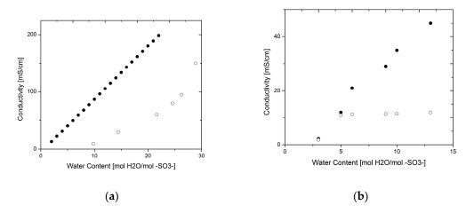
**Figure 3.** Effect of geometry: (a) Springer et al. [30] in-plane ( $\bullet$ ) vs. Alberti et al. [25] through-plane ( $\bigcirc$ ); (b) Lee et al. 2-probe ( $\bullet$ ) vs. 4-probe measurements ( $\bigcirc$ ) [12].
