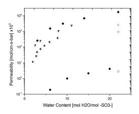
**Figure 4.** Water permeability. Ise, Kreuer at 27 °C (•) [31]; Rivin et al. at 32 °C (□) [1]; Zhao et al. at 70 °C (◊) [8]; Majztrik et al. at 80 °C (×) [9]; Zawodinski et al. at 30 °C (•) [23]; Zhao et al. at 70 °C (•) [8]; Edmondson et al. at room temperature ( $\mathbf{v}$ ) [22].
