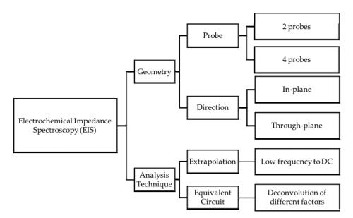
Figure 1. Electrochemical Impedance Spectroscopy: measurement and analysis techniques.
