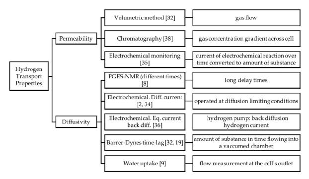
Figure 5. Permeability and Diffusivity measuring techniques.
