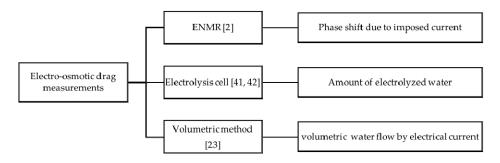
Figure 7. Electro-osmotic drag measuring techniques.
