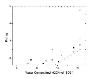
**Figure 8.** Electro-osmotic drag data compilation. Ise, Kreuer at 27 °C (**■**) [31]; Kreuer et al. at 27 °C ( $\bigtriangledown$ ) [40]; Springer et al. at 80 °C ( $\bigcirc$ ) [30]; Onda et al. at 80 °C ( $\times$ ) [42]; Kreuer et al. at 80 °C (+) [2]; Zawodinski at 30 °C (**v**) [23].
