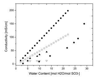
Figure 2. Nafion<sup>™</sup> 117 conductivity value comparison. Springer et al. at 80 °C, in-plane, 2-probe
