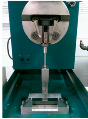
Figure 6. Experimental setup of the three-point bending test.
