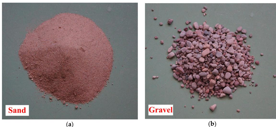
Figure 3. Aggregates used in the studies: (a) Sand; (b) gravel.
