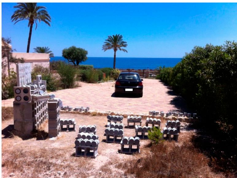
**Figure 2.** Image of the samples placed in the exposure station of Santa Pola's Cape (province of Alicante). As can be observed, the distance from the Mediterranean Sea is about 100 m.
