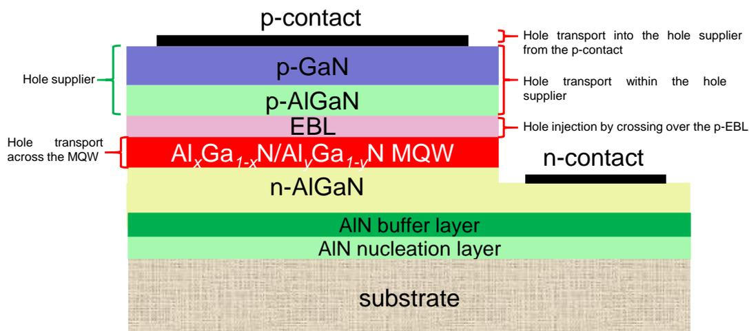
**Figure 1.** Schematic device architecture for a typical AlGaIn based DUV LED and the four key factors that co-decide the hole injection efficiency. The hole supplier contains the p-AlGaIn layer and the p-GaN layer.
