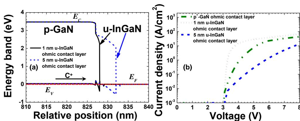
**Figure 2.** (a) Energy band diagrams at the equilibrium state for u-InGaN/p-GaN structures with the u-InGaN layer thicknesses of 1 nm and 5 nm, respectively; (b) calculated current in terms of the applied voltage for LEDs with p<sup>+</sup>-GaN, 1 nm thick u-InGaN and 5 nm thick u-InGaN as the ohmic contact layers, respectively. Here, u-InGaN,  $E_C$ ,  $E_V$  and  $E_F$  represent the undoped InGaN cap layer, the conduction band, the valence band and the Fermi level, respectively.
