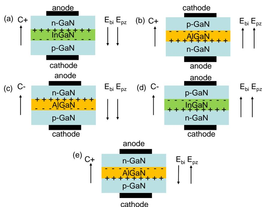
**Figure 3.** (a) [0001] oriented n-GaN/InGaN/p-GaN polarization tunnel junction; (b) [0001] oriented p-GaN/AlGaN/n-GaN polarization tunnel junction; (c) [00-1] oriented n-GaN/AlGaN/p-GaN polarization tunnel junction; (d) [000-1] oriented p-GaN/InGaN/n-GaN polarization tunnel junction and (e) [0001] oriented dielectric-constant-controlled (DCC) tunnel junction.  $E_{bi}$ ,  $E_{pz}$  represent the built-in electric field and the polarization induced electric field, respectively.
