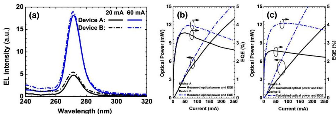
**Figure 8.** (a) Experimentally measured EL spectra; (b) experimentally measured EQE and optical power, and (c) numerically calculated EQE and optical power for Devices A and B, respectively. Reproduced from Ref. [24], with the permission of American Chemical Society.
