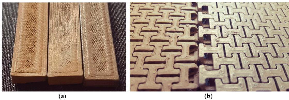
**Figure 12.** Example of Bronzefill samples: (a) Bending test specimens without polishing (left), polished with a steel brush (middle) and by inserting the specimen in a rotating drum filled with small screws (right), sample widths of 10 mm; (b) Chainmail (for an overview image, cf. Figure 11) before (left sample) and after polishing in a rotating drum (right sample), chain link width of 12 mm.
