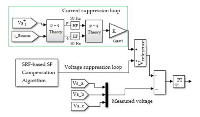
Figure 9. The proposed control algorithm for the SF.
