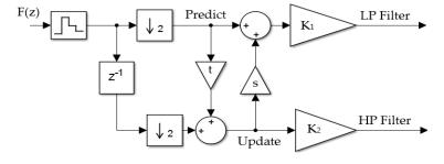
**Figure 3.** Schematic of lifting wavelet transform.
