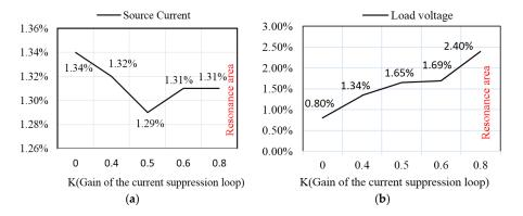
**Figure 16.** The THD (in percent) when the proposed SRF method equipped with the improved SF is under an unbalanced inductive load: (a) Grid-end currents; and (b) load-terminal voltages.
