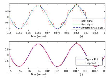
**Figure 5.** The orthogonal signals generator: (a) comparison between ideal signal and produced sine signal using wavelet-based PLL; (b) comparison of produced sine signals using the proposed PLL and a typical PLL.
