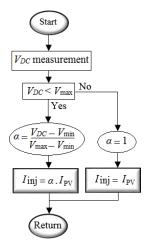
Figure 10. Proposed controller to regulate the DC-link voltage.
