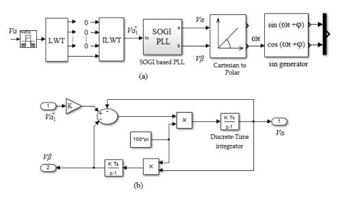
**Figure 4.** Block diagram of: (a) Wavelet-based signals generator; (b) internal structure of the SOGI-based phase locked loop (PLL).
