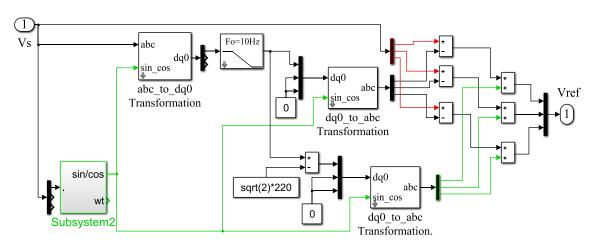
**Figure 7.** Proposed synchronous reference frame (SRF)-based compensation algorithm for the series filter (SF). Vref: voltage references.
