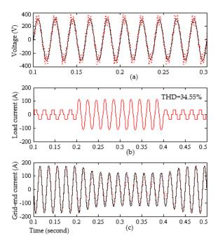
**Figure 15.** (a) Power grid and load voltages (V); (b) the load-terminal current (A) (phase a) (THD = 34.55%); and (c) power grid-end currents (A), compensated for by the proposed SRF method (THD = 1.29%) and compensated for by the SRF method [29].
