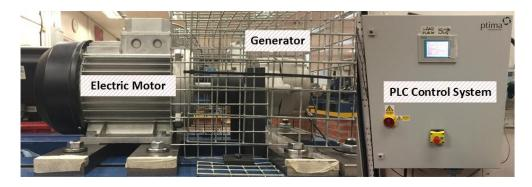
Figure 7. View of experimental generator test set up.
