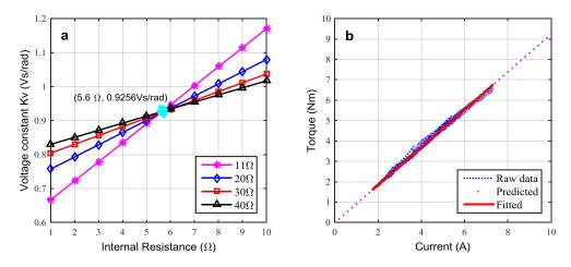
**Figure 5.** (a) Online voltage constant coefficient vs internal resistance; (b) online fitted torque constant coefficient,  $k_{\rm T}$ .
