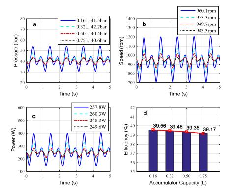
**Figure 17.** (a) Measured motor pressure; (b) measured shaft speed; (c) measured regenerative power; (d) measured power regeneration efficiency, at 0.16 L, 0.32 L, 0.50 L and 0.75 L accumulator capacity.
