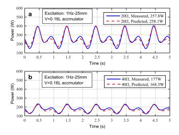
**Figure 14.** Predicted and measured power at (a) 20  $\Omega$  load resistance; (b) 40  $\Omega$  load resistance.
