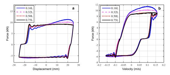
**Figure 20.** (a) Measured displacement-force loops; (b) measured velocity-force loops, at 0.16 L, 0.32 L, 0.50 L and 0.75 L accumulator capacities.
