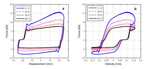
**Figure 15.** (a) Measured displacement-force loops; (b) measured velocity-force loops, at 11  $\Omega$ , 20  $\Omega$ , 30  $\Omega$  and 40  $\Omega$  load resistances.
