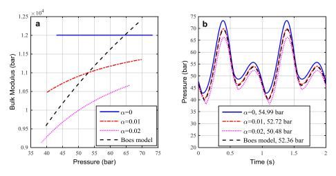
Figure 9. (a) Bulk modulus variation with motor pressure; (b) predicted motor pressures for different bulk modulus values.
