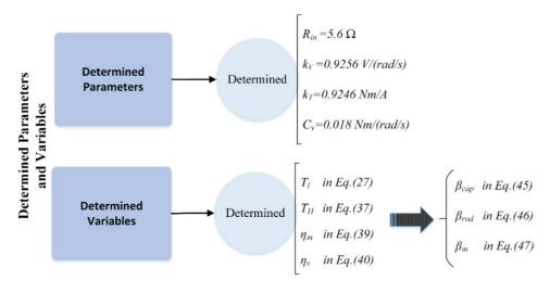
Figure 10. Determined parameters and variables in power regeneration unit and hydraulic system.
