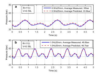
**Figure 11.** Predicted and measured pressure at (a) 0.5 Hz frequency and 25 mm amplitude; and (b) 1.0 Hz frequency and 20 mm amplitude (R is equal to the external load  $R_L$  and V is the same as accumulator capacity  $V_c$ ).
