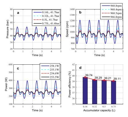
**Figure 16.** (a) Predicted motor pressure; (b) predicted shaft speed; (c) predicted regenerative power; (d) predicted power regeneration efficiency, at 0.16 L, 0.32 L, 0.50 L and 0.75 L accumulator capacities.
