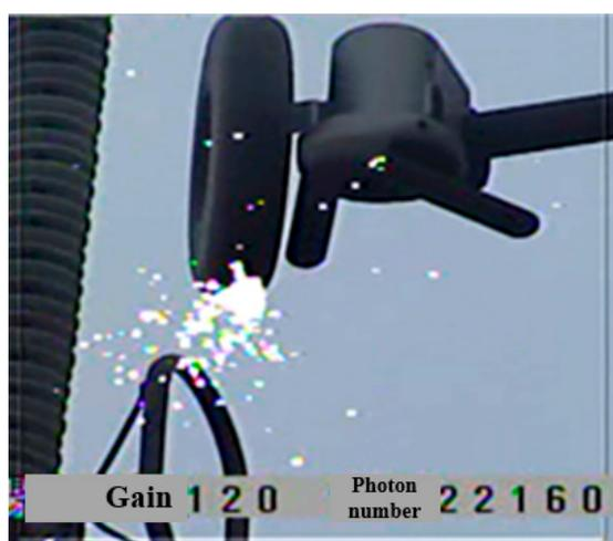
**Figure 14.** Detection image of Type A in the on-site test.**Table 7.** Photon numbers of Type A in the on-site test.
