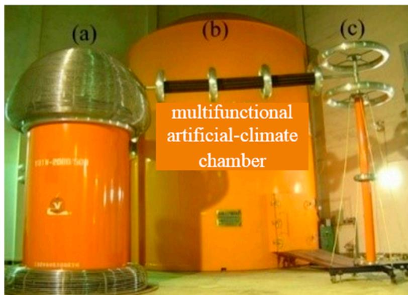
**Figure 1.** Experimental facilities (a) 500 kV/2000 kVA testing transformer; (b) multifunctional artificial-climate chamber; (c) 500 kV capacitive voltage divider.
