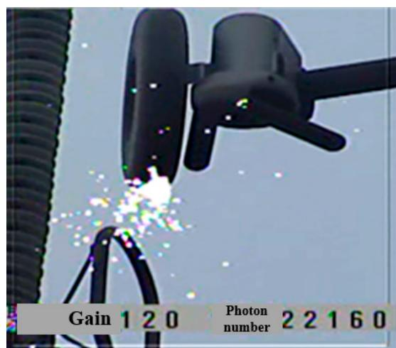
**Figure 14.** Detection image of Type A in the on-site test.**Table 7.** Photon numbers of Type A in the on-site test.
