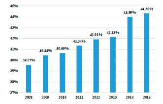
Figure 3. Average thermal efficiency of power plants in China (2008–2015).
