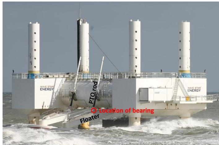
**Figure 2.** Wavestar prototype located at Hanstholm (Denmark) showing the location of the investigated bearing. Power take-off: PTO.
