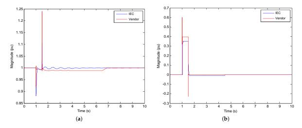
**Figure 8.** Type IIIB results. Simulation scenario: p = 1.0 pu, u = 0.85 pu, t = 500 ms,  $w_s = 1.1$ . (a) Active power, p; and (b) reactive current,  $i_q$ .
