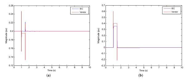
**Figure 6.** Type IIIB results. Simulation scenario: p = 0.20 pu, u = 0.85 pu, t = 500 ms. (**a**) Active power, *p*; and (**b**) reactive current,  $i_q$ .
