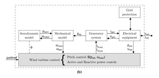
**Figure 1.** Configuration of a Type IIIB wind turbine. (**a**) Main elements; and (**b**) corresponding model block diagram. WT: wind turbine; and WTT: wind turbine terminals.
