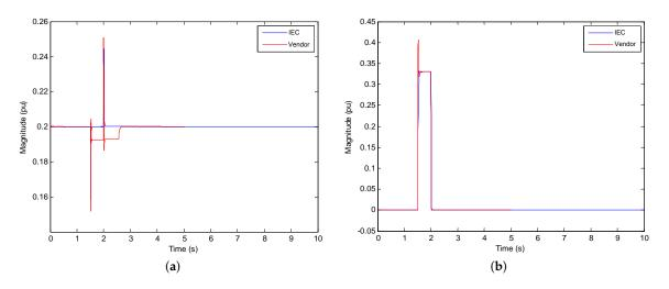
**Figure 12.** Type IVA results. Simulation scenario: p = 0.20 pu, u = 0.85 pu, t = 500 ms. (a) Active power, p; and (b) reactive current,  $i_q$ .
