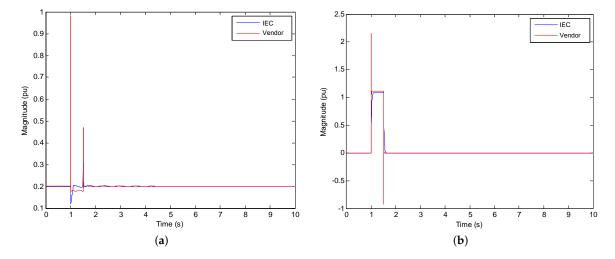
**Figure 5.** Type IIIB results. Simulation scenario: p = 0.20 pu, u = 0.50 pu, t = 500 ms. (a) Active power, p; and (b) reactive current,  $i_q$ .
