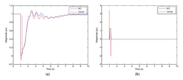
**Figure 7.** Type IIIB results. Simulation scenario: p = 1.0 pu, u = 0.20 pu, t = 200 ms,  $w_s = 1.1$ . (a) Active power, p; and (b) reactive current,  $i_q$ .
