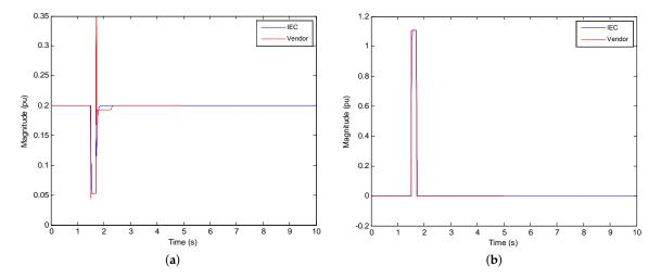
**Figure 10.** Type IVA results. Simulation scenario: p = 0.20 pu, u = 0.20 pu, t = 200 ms. (a) Active power, p; and (b) reactive current,  $i_q$ .
