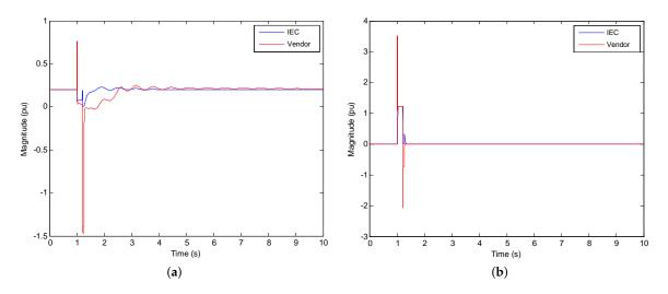
**Figure 4.** Type IIIB results. Simulation scenario: p = 0.20 pu, u = 0.20 pu, t = 200 ms. (a) Active power, p; and (b) reactive current,  $i_q$ .
