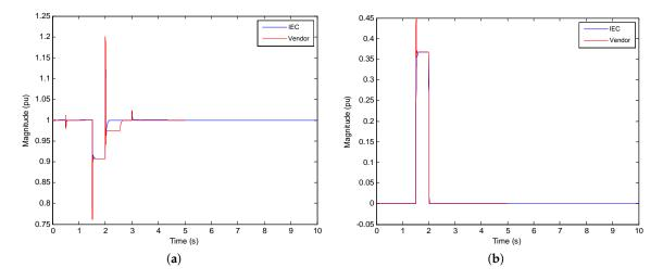
**Figure 15.** Type IVA results. Simulation scenario: p = 1.0 pu, u = 0.85 pu, t = 500 ms. (a) Active power, p; and (b) reactive current,  $i_q$ .
