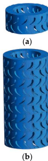
Figure 7. Simulation model of the turbodrill blade. (a) Single-stage blade model; (b) Multi-stage and multi-blade model.
