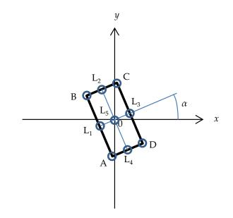
**Figure 1.** Definition of wind direction  $\alpha$  and representative locations on the roof. Circles indicate the representative locations, which are corners A–D, midpoints of an edge L<sub>1</sub>–L<sub>4</sub>, and center L<sub>5</sub>.
