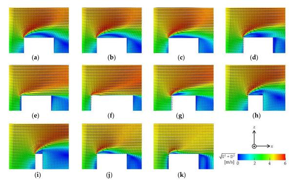
**Figure 6.** Vertical distributions of the wind vectors along the dotted lines indicated in Figure 5. (a) Line i; (b) Line ii; (c) Line iii; (d) Line iv; (e) Line v; (f) Line vi; (g) Line vii; (h) Line viii; (i) Line ix; (j) Line x; (k) Line xi.
