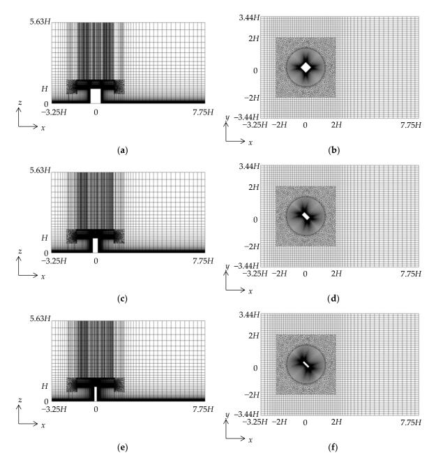
**Figure 2.** Computational domains and grids. (a) Vertical cross section for run case  $100_{450}$  at y = 0; (b) Horizontal cross section for run case  $100_{450}$  at z = 0; (c) Vertical cross section for run case  $050_{450}$  at y = 0; (d) Horizontal cross section for run case  $050_{450}$  at z = 0; (e) Vertical cross section for run case  $025_{450}$  at y = 0; (f) Horizontal cross section for run case  $025_{450}$  at z = 0. Here, H (=0.16 m) is the height of the building.
