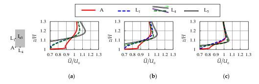
**Figure 11.** Vertical profiles of horizontal wind velocity ratios at representative locations on the roof, in the case of no prevailing wind direction. (**a**) HAR = 1.00; (**b**) HAR = 0.50; (**c**) HAR = 0.25.
