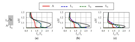
**Figure 12.** Vertical profiles of turbulence intensity rations at representative locations on the roof, in the case of no prevailing wind direction. (a) HAR = 1.00; (b) HAR = 0.50; (c) HAR = 0.25.
