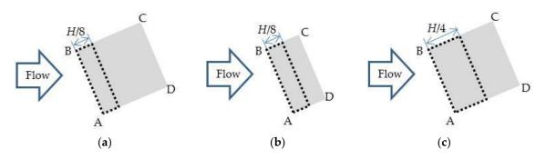
**Figure 7.** Top view of the windward quarter and windward half of the roof. (**a**) Windward quarter, HAR = 1.00; (**b**) Windward half, HAR = 0.50; (**c**) Windward half, HAR = 1.00.
