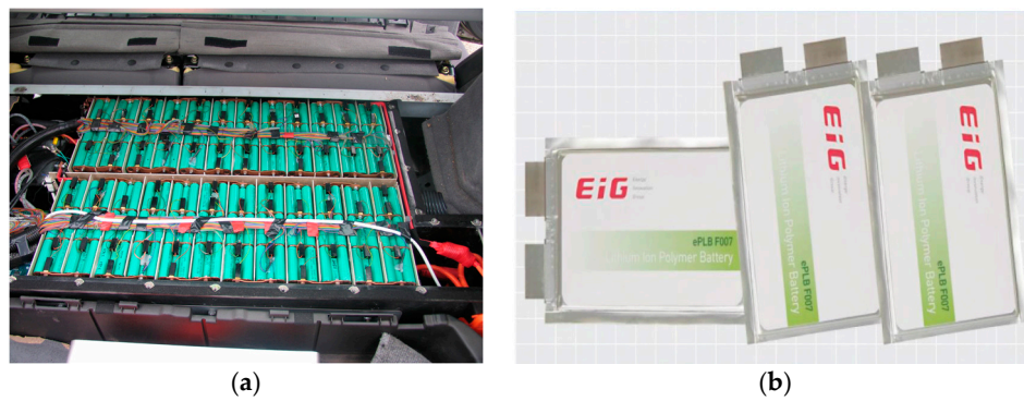
Figure 2. Second-life battery cells/blocks: (a) battery blocks (32.4 Ah) that used in plug-in hybrid electric vehicle (PHEV) for more than five years; and (b) battery cells EIG (7 Ah).
