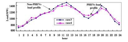
Figure 3. The influence of PHEVs on load curve in smart grid.
