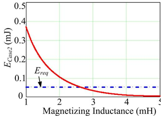
**Figure 12.** Available energy in Case 2 vs. magnetizing inductance.
