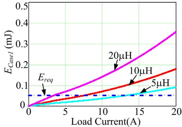
**Figure 11.** Available energy in Case 1 vs. load current.
