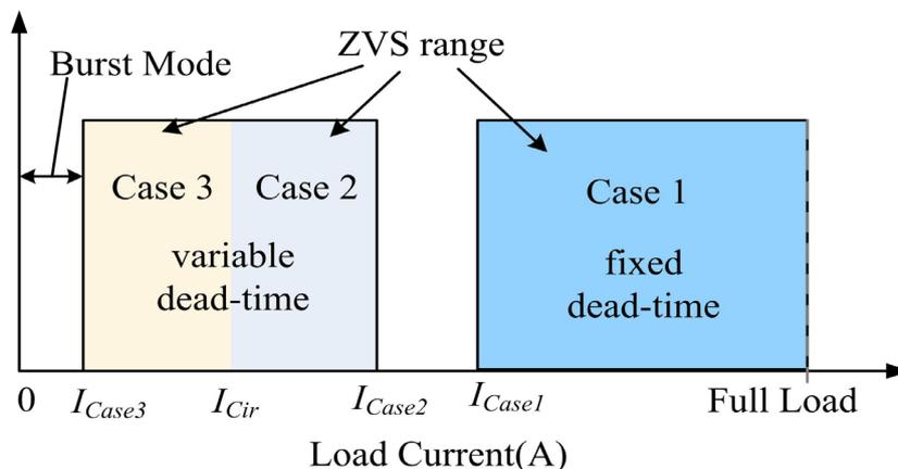
**Figure 15.** Operational modes with the variable dead-time control.
