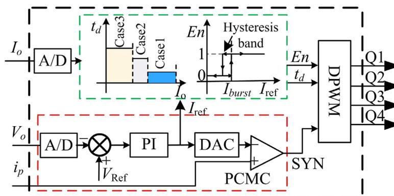
Figure 17. Control block diagram of the proposed method.
