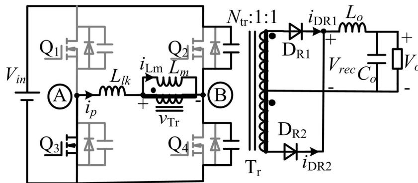
Figure 5. Equivalent circuit in Case 1.
