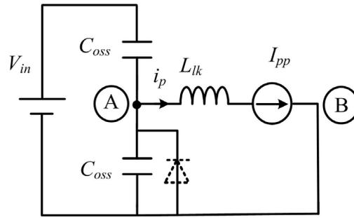
Figure 4. Simplified circuit during  $[t_0, t_1]$ .
