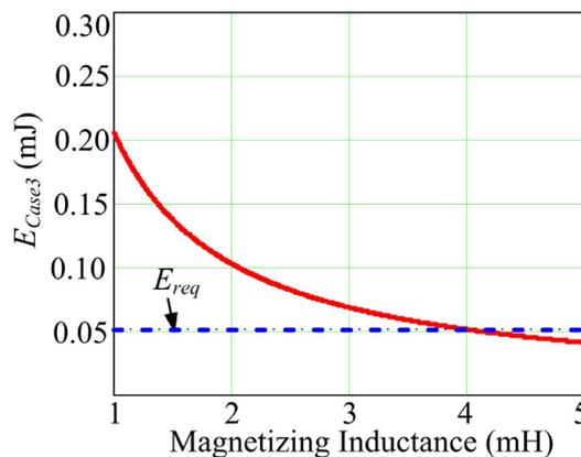
**Figure 13.** Available energy in Case 3 vs. magnetizing inductance.
