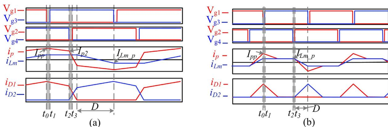
**Figure 2.** Key waveforms in different modes: (a) Continuous current mode (CCM); (b) Discontinuous current mode (DCM).
