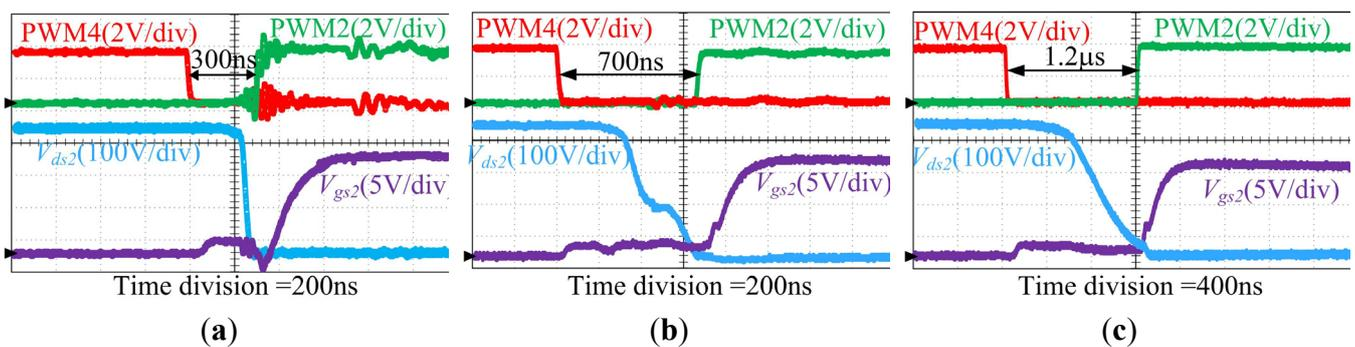
**Figure 19.** Experimental waveforms of  $Q_2$  under different load conditions. (a) Case 1,  $I_o = 20$  A; (b) Case 2,  $I_o = 5$  A; (c) Case 3,  $I_o = 0.5$  A.
