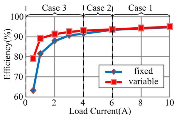
**Figure 20.** Measured efficiencies with different control methods.
