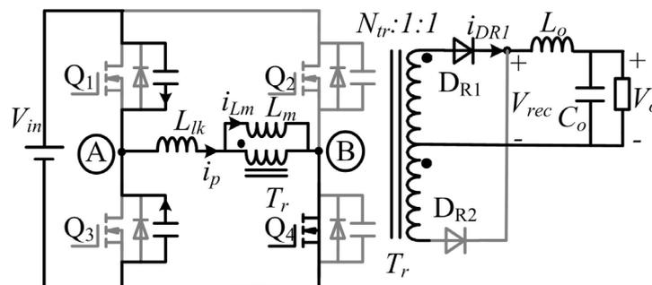
Figure 3. Equivalent circuit during  $[t_0, t_1]$ .
