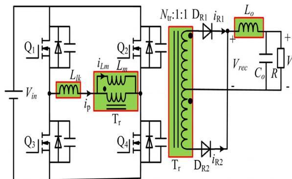
**Figure 1.** Circuit diagram of a phase-shifted full-bridge (PSFB) converter.
