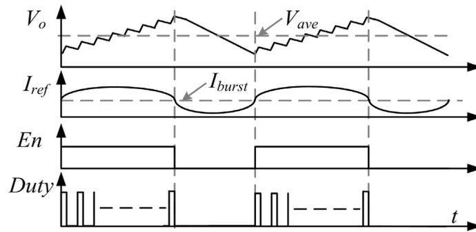
**Figure 18.** Key waveforms with burst mode control.
