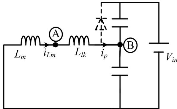
Figure 10. Simplified circuit in Case 3.
