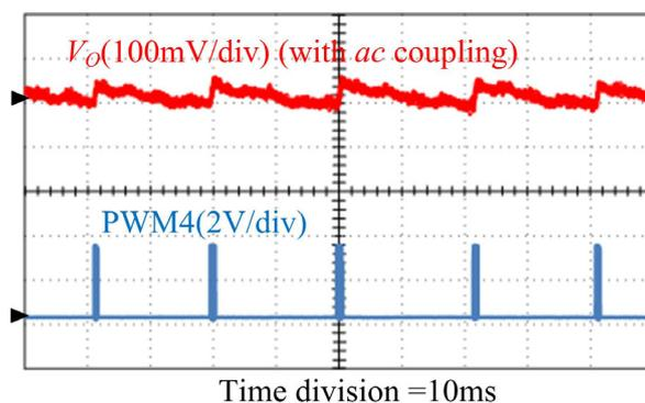
**Figure 21.** Key waveforms under standby condition.
