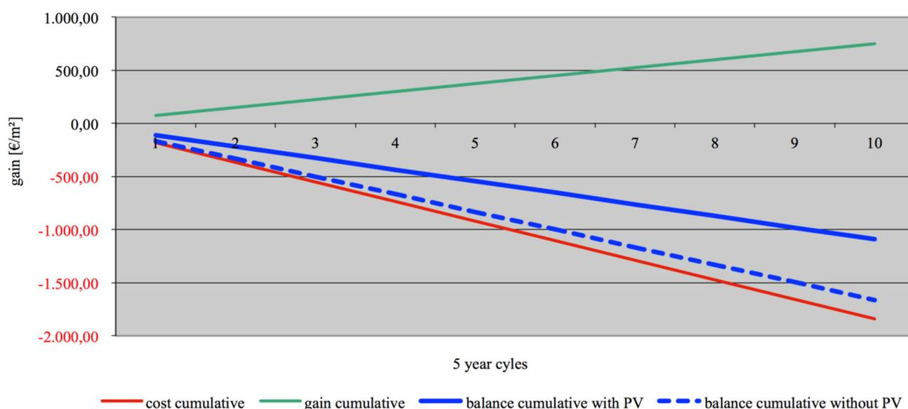
**Figure 3.** Lifecycle costs of a conventional façade with high value cladding and a BIPV façade over a period of 50 years divided in 5-year cycles.
