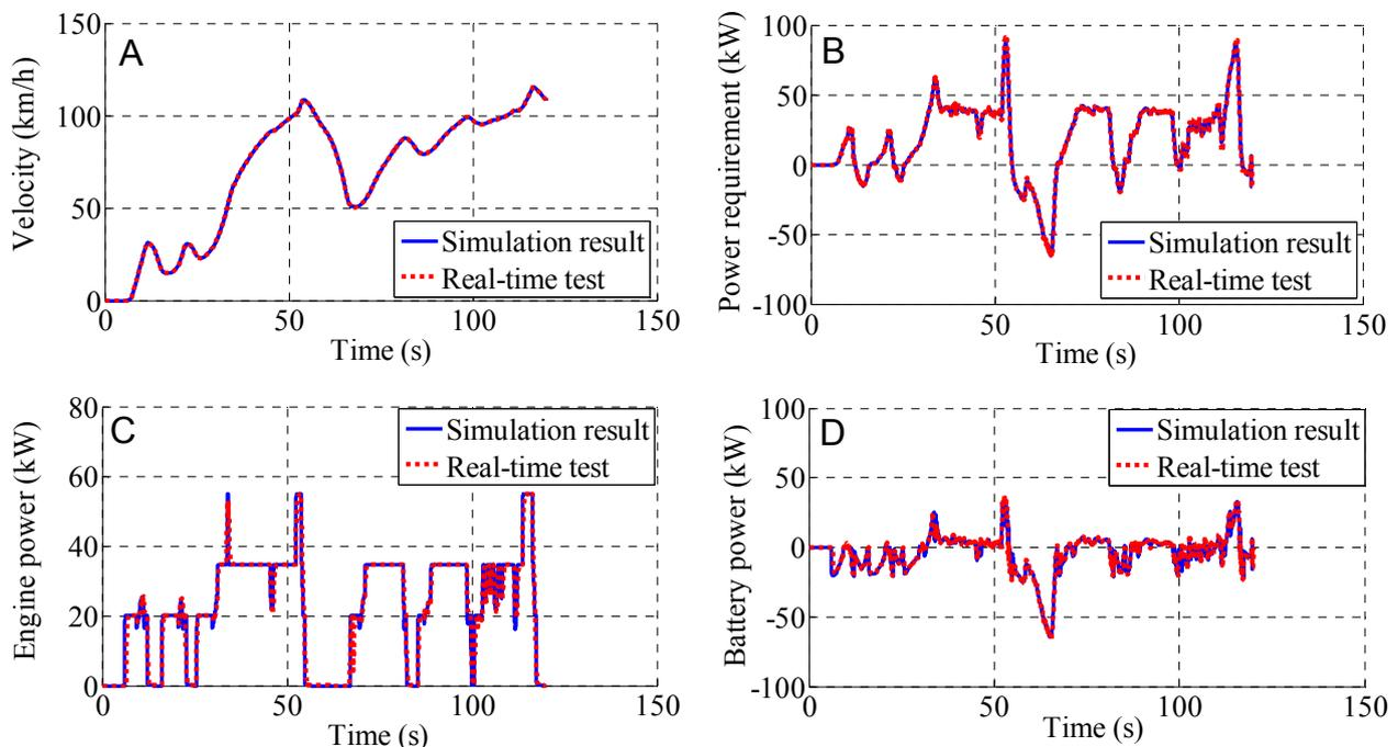
**Figure 10.** Comparison results of driver-in-the-loop real-time test and offline simulation: (A) Velocity; (B) Required power; (C) Engine power; (D) Battery power.
