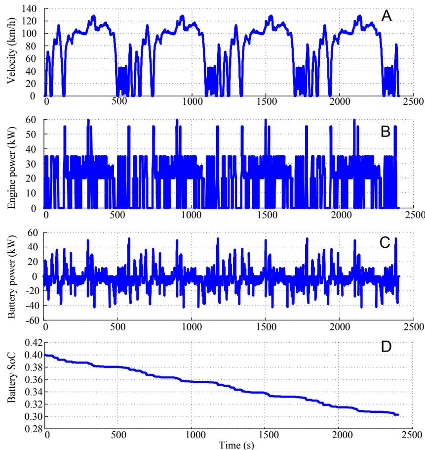
**Figure 4.** Simulation results based on the proposed strategy: (A) Velocity *versus* time; (B) Engine power *versus* time; (C) Battery power *versus* time; (D) Battery SoC *versus* time.
