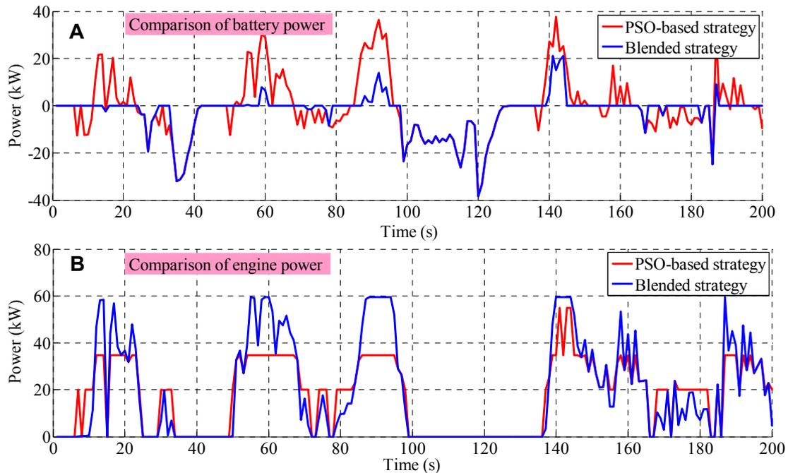
**Figure 5.** Simulation result of power allocation: (A) Battery power; (B) Engine output power.
