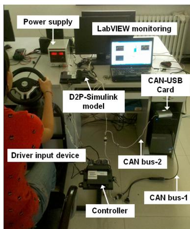
**Figure 8.** Driver-in-the-loop experiment platform.
