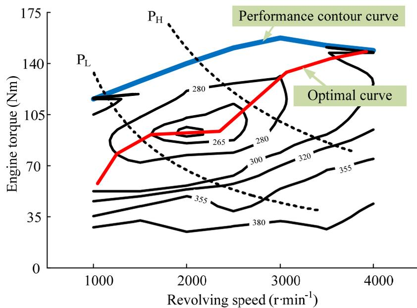
**Figure 2.** Efficiency map of the engine system.
