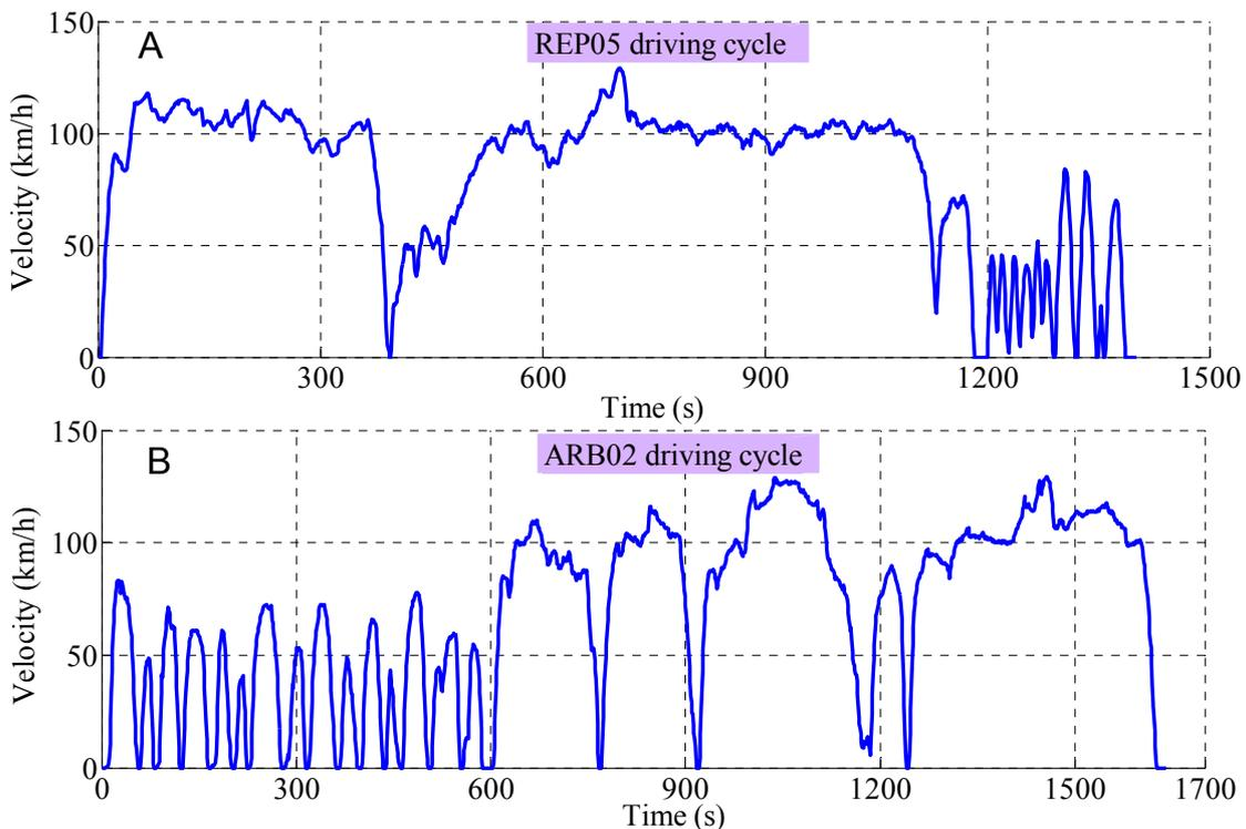
**Figure 6.** Test driving cycles: (A) Profiles of REP05; (B) Profiles of ARB02.
