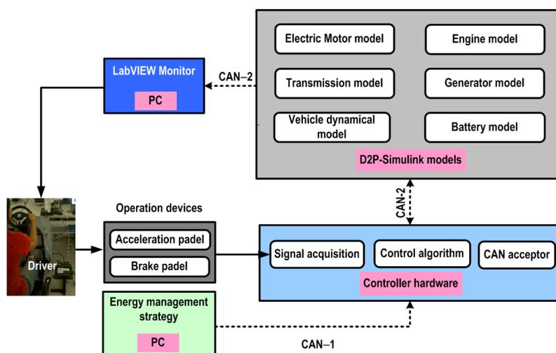
**Figure 7.** Schematic diagram of driver-in-the-loop experiment platform.
