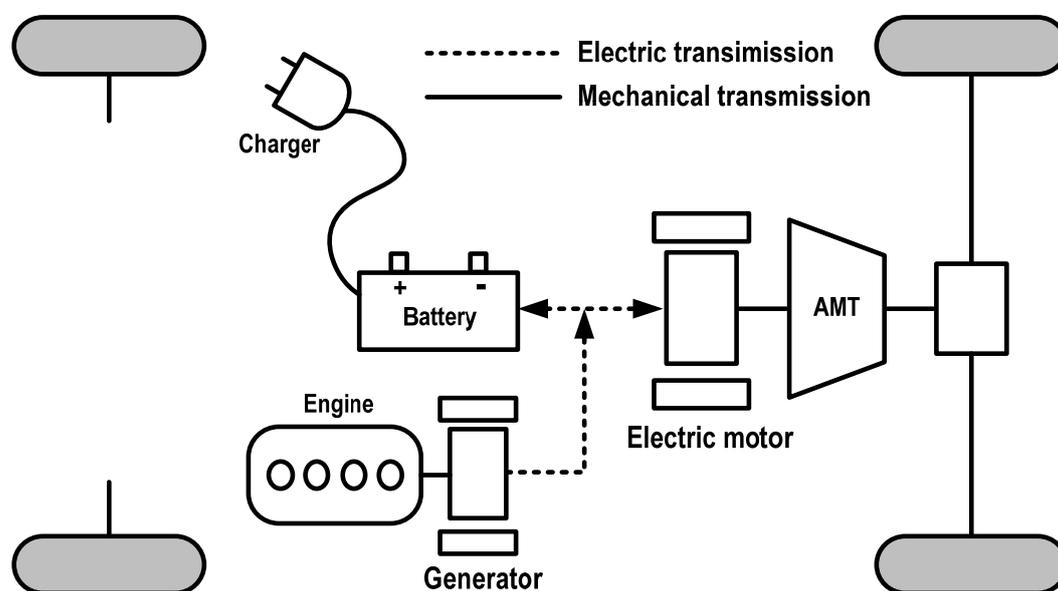
**Figure 1.** Schematic diagram for powertrain system of plug-in hybrid electric vehicle (PHEV).
