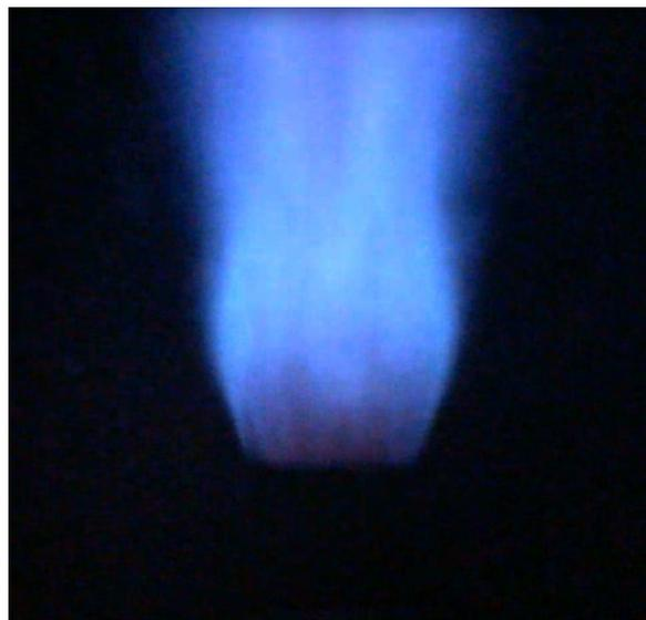
**Figure 2.** Photography of hydrogen-enriched methane flame stabilized behind the lance of the PPBB burner.
