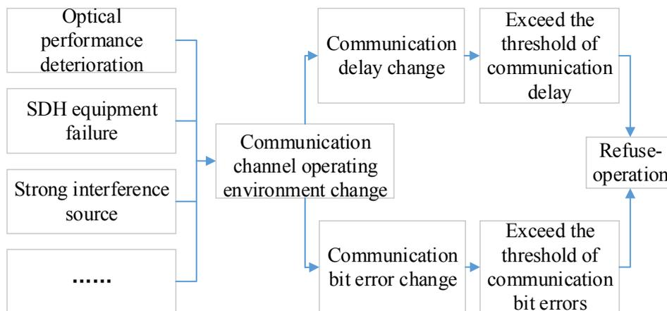
**Figure 10.** The progress of refuse-operation.
