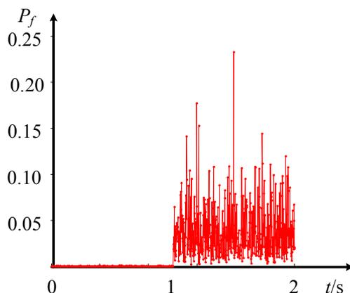
**Figure 17.** Real time false trip probability for inconsistent delay.
