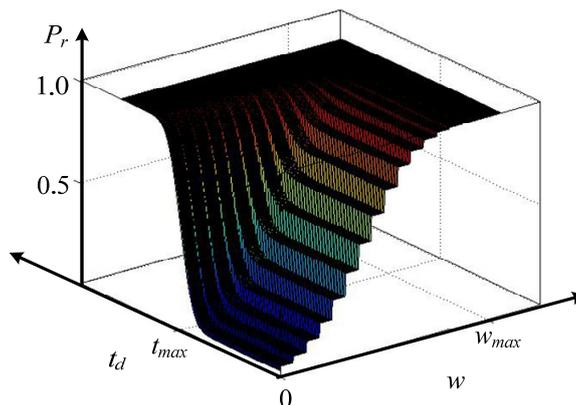
**Figure 11.** Refuse-operation probability for consistent delays and bit errors.
