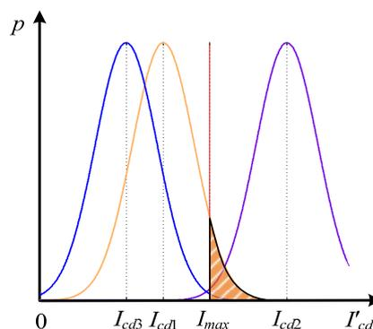
**Figure 3.** The probability density function of the differential current.
