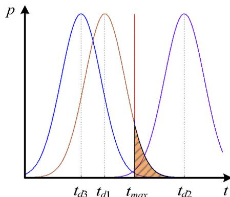
**Figure 6.** The probability density function of the consistent delay.
