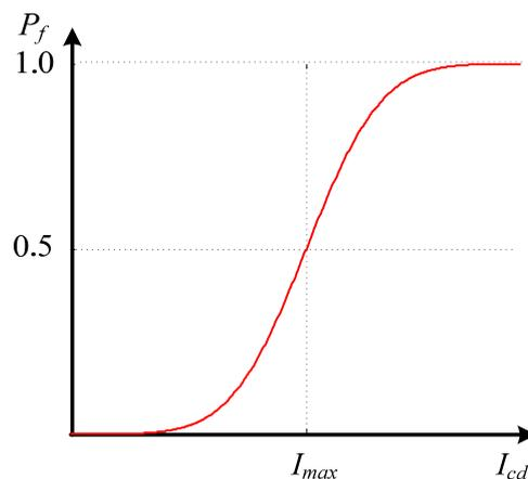
**Figure 4.** False trip probability caused by the differential current.
