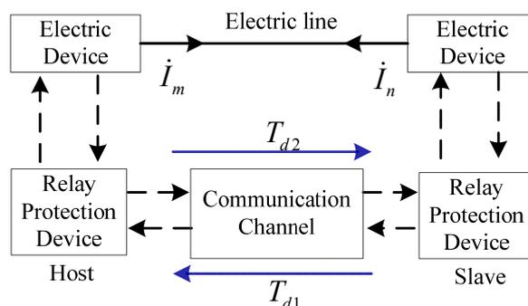
Figure 1. Signal transmission in current differential protection.
