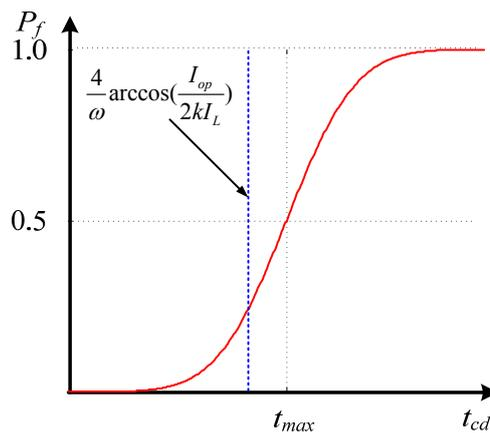
**Figure 5.** False trip probability follows the first form of braking ratio criterion and start criterion.
