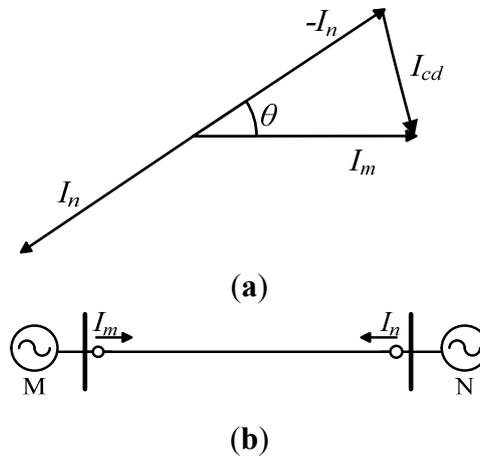
**Figure 2.** Current vector changes caused by inconsistent delay. (a) Vector diagram of currents; (b) current differential protection.
