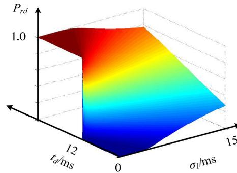
**Figure 13.** Refuse-operation probability considering consistent delay distribution.
