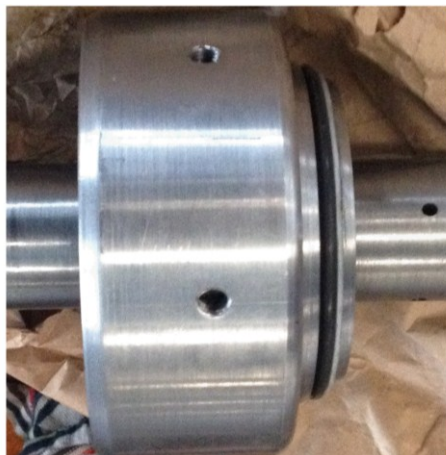
Figure 3. Hydraulic piston with T-shaped channels.
