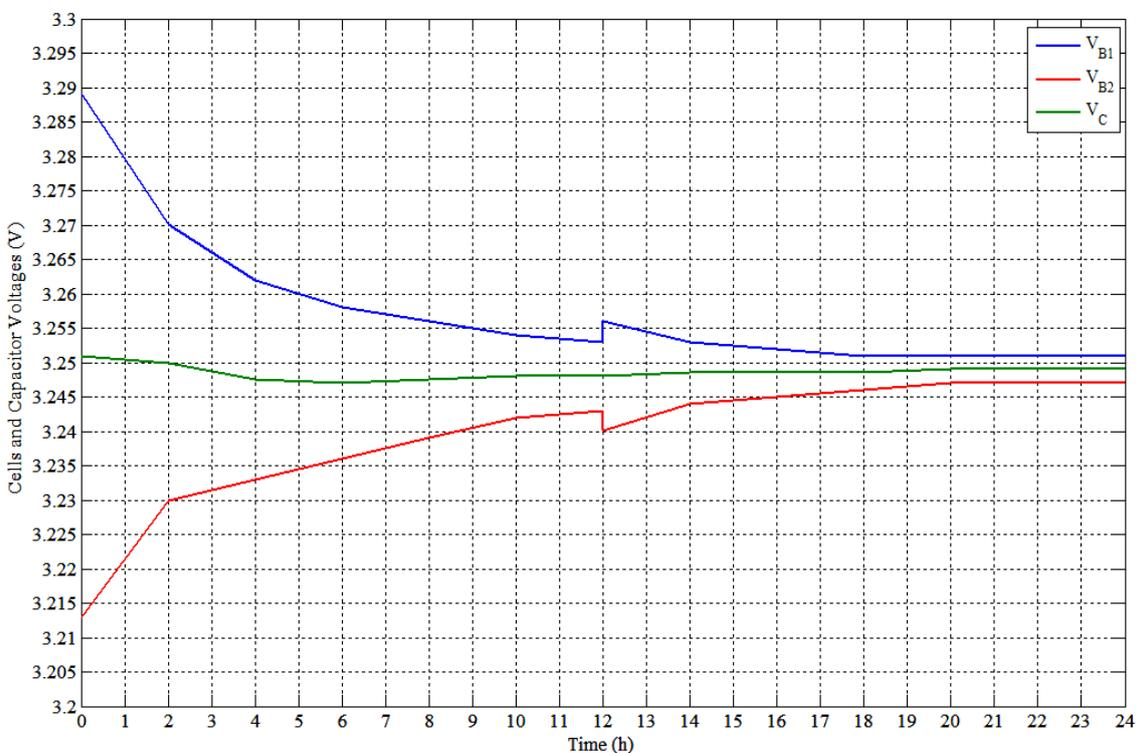
**Figure 28.** Experimental results of 2.3 A·h cells with SSC balancing (Test No. 3).
