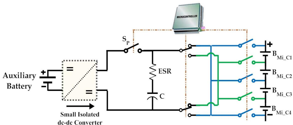
Figure 5 shows the model of one SSC-IMB. The model consists of: four cells of the module, AB (for the SSC capacitor boosting), balancing capacitor, switching devices, and the controller. As shown in Figure 5, the SSC-MIB can be described as follows:
