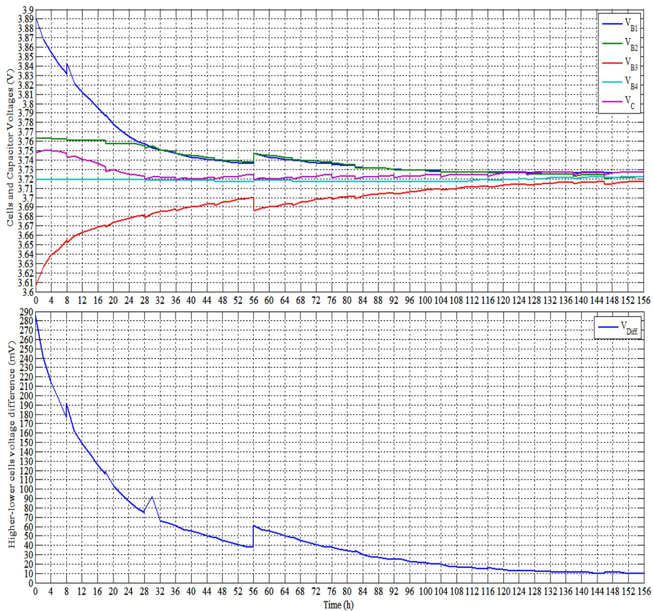
**Figure 36.** Experimental results of 20 A·h cells with between modules converter balancing Test No. 3 (top to bottom), the two modules' cells voltages, modules voltages, modules voltages screen capture.
