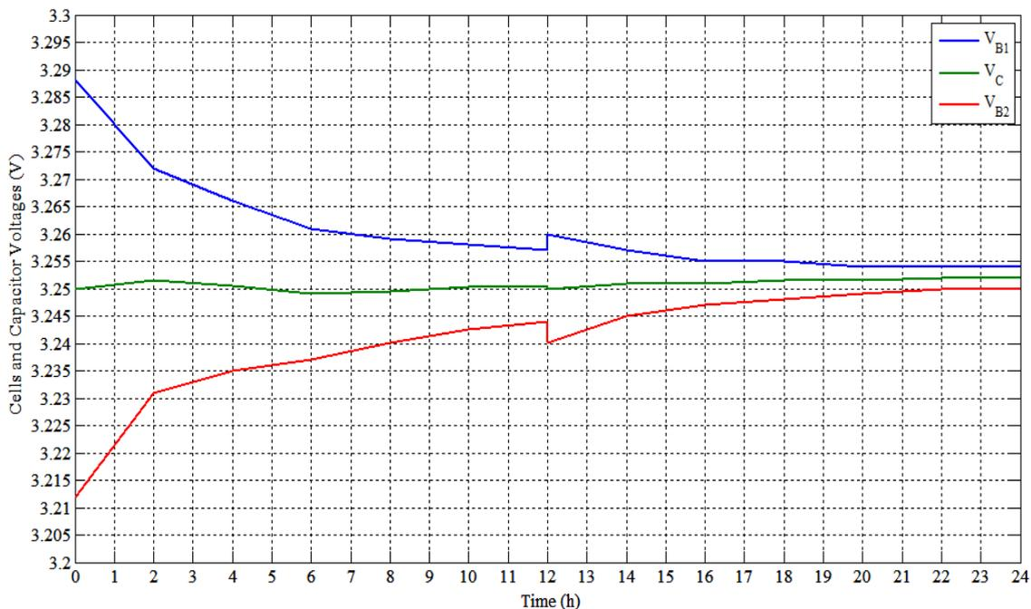
**Figure 27.** Experimental results of 2.3 A·h cells with SSC balancing (Test No. 2).
