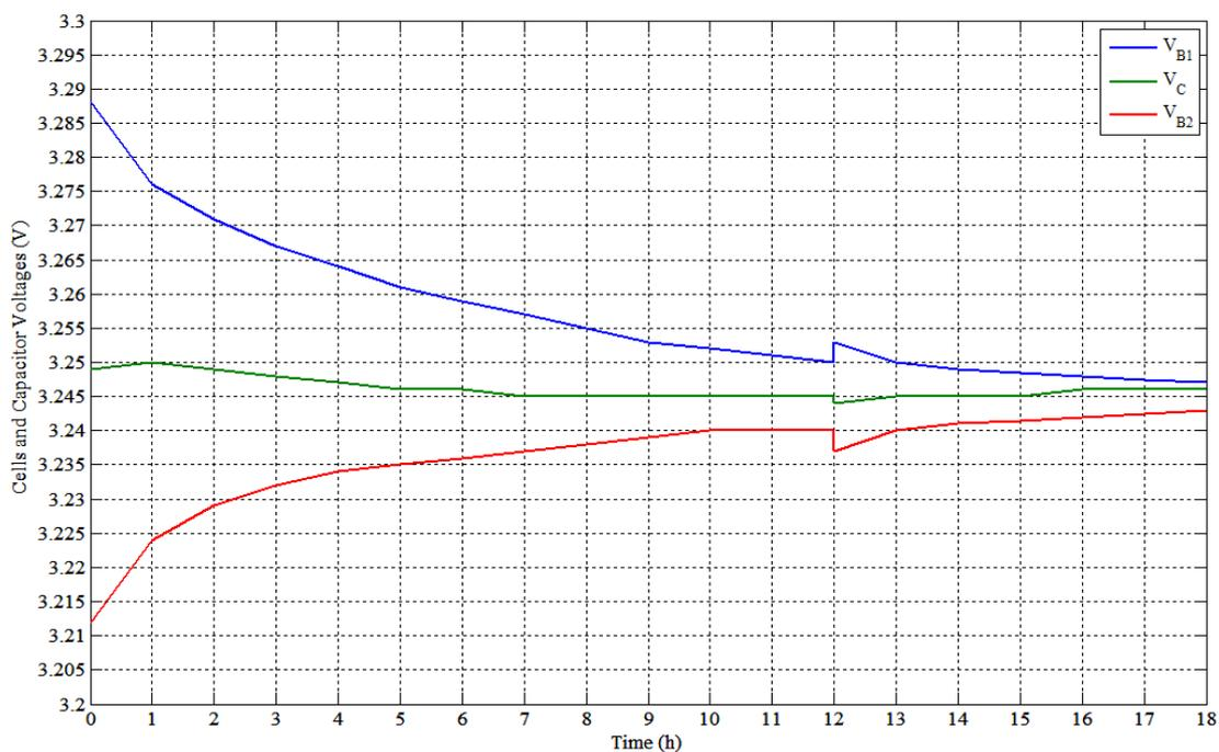
**Figure 30.** Experimental results of 2.3 A·h cells with SSC balancing (Test No. 5).
