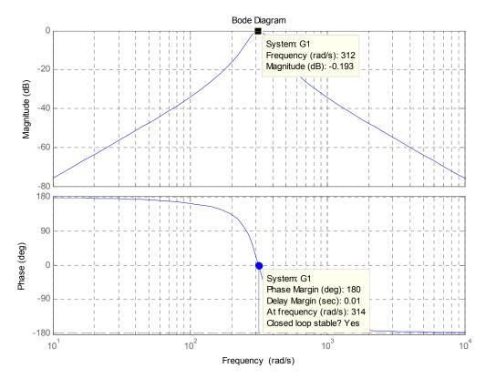
**Figure 4.** Bode diagram of the proposed band-pass filter.
