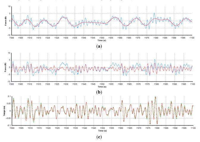
The reconstructed low frequency component of surge is then added in time domain to the recorded high frequency part to provide the overall surge response time series, on which the following data analysis is based.
