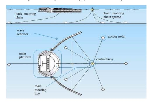
Figure 2. Conceptual mooring system of Wave Dragon.
