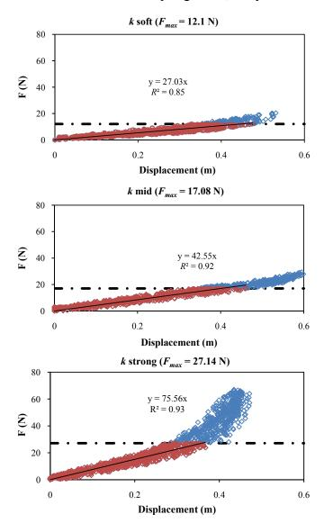
These values have been confirmed by the F-D curve obtained in irregular waves, as shown in Section 3.4. To distinguish between the two, the former—derived from the calibration—are referred to as "target" stiffness, the latter—experienced during the test—as "actual" stiffness. However, given their
