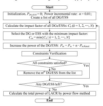
Figure 4. Block diagram of calculating the power supply capacity of the LACR.
