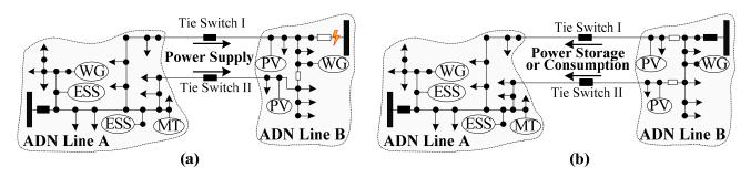
In Figure 3 there is more than one tie switch between the ADN lines, and the power supply and storage capacity is the maximum summation of the power transmitted by all the tie switches. If there is no adjacent line, the power supply and storage capacity of ADN line is 0.
