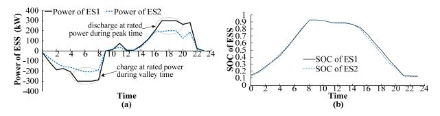
As shown in Figure 8, ES1 and ES2 charge during [0,8], and discharge during [10,23], maximizing the benefits of charging/discharging at different electricity prices. The discharging power reaches the rated ESS discharging power during the peak time, and the charging power reaches the rated charging power during the valley time, maximizing the energy of peak shaving.
