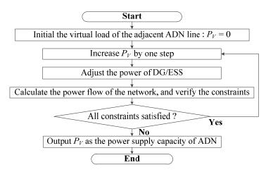
The process of the algorithm is shown in Figure 5. The iteration process of computing the power storage capacity of an ADN line is similar to that of power supply capacity, while a difference exists in
