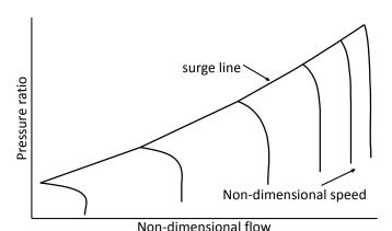
Figure 5. Schematic compressor map.
