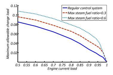
It can be seen that engine allowable change load will be decreased when the engine gets closer to its full load condition. Additionally, in high engine loads, where the temperature controller limits the maximum allowable change load, the steam injection can enhance the gas turbine performance. This is
