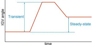
There is no problem with current control logic until the turbine is near full load condition. Near full load, the IGVs are almost fully open and this means that the controller doesn't have the needed reserve
