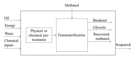
Figure 3. Major steps involved in the industrial phase of biodiesel production.
