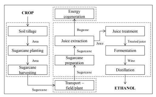
Figure 5. System boundaries for anhydrous ethanol production.
