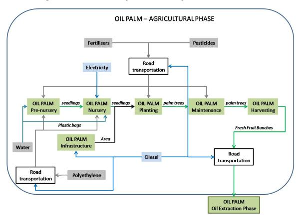
Figure 1. Flowchart of the production of oil palm fresh fruit bunches.
