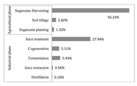
Figure 6. Relative costs per stage of anhydrous ethanol production.
