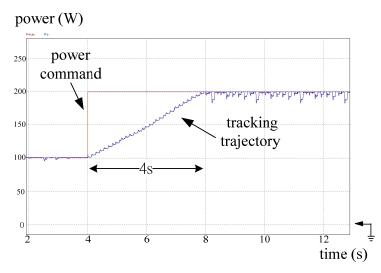
**Figure 19.** Simulated result: tracking trajectory of the converter with the DLAA while PV power steps up from 100 to 200 W. Note: power: 50 W/div; time: 1 s/div.
