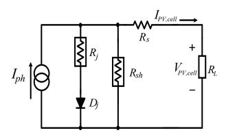
From the characteristics of a p-n junction and the equivalent circuit, output current of PV arrays,  $I_{PV}$ , can be described as:
