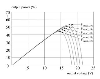
**Figure 3.**  $P_{PV}-V_{PV}$  curves of the PV module with fixed irradiation (1000 W/m<sup>2</sup>).
