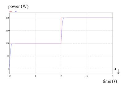
To examine the step-down change, Figures 20 and 21 show the simulated results of the PV converter with the POM and with the DLAA, respectively. The transition time is 6 s in Figure 20 and 50 ms in Figure 21. In hardware illustration, Figure 22 is the output power measurement of the converter with the POM in the case of the PV power changing from 100 W to 200 W while Figure 23 shows the measured result with the DLAA.
