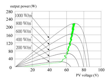
Figure 11. The MPPT trajectory by the DLAA under fixed temperature.
