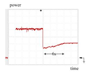
**Figure 25.** Practical measurement: tracking trajectory of the converter with the DLAA while PV power steps down from 200 to 100 W. Note: power: 50 W/div; time: 0.5 s/div.
