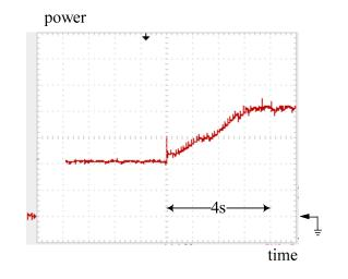
**Figure 23.** Practical measurement: tracking trajectory of the converter with the DLAA while PV power steps up from 100 to 200 W. Note: power: 50 W/div; time: 0.5 s/div.
