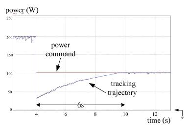
**Figure 21.** Simulated result: tracking trajectory of the converter with the DLAA while PV power steps down from 200 to 100 W. Note: power: 50 W/div; time: 1 s/div.
