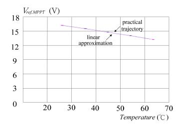
Figure 6. The trajectory of  $V_{\text{ref, MPPT}}$  versus temperature T.
