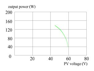
Figure 15. MPPT trajectory by the DALL while irradiation and temperature increase.
