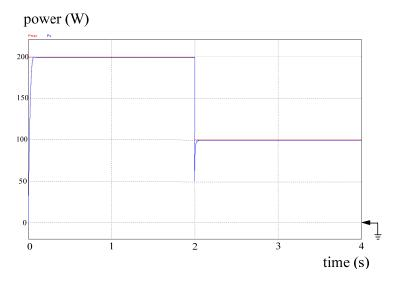
**Figure 22.** Practical measurement: tracking trajectory of the converter with the POM while PV power steps up from 100 to 200 W. Note: power: 50 W/div; time: 1 s/div.
