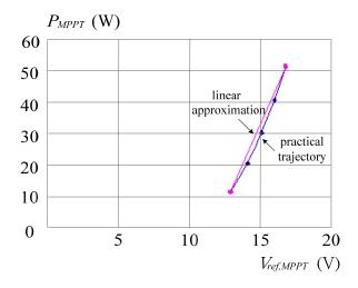
**Figure 5.** The relationship between  $P_{\text{MPPT}}$  and  $V_{\text{ref,MPPT}}$  while module temperature increases from 25 to 65 °C.
