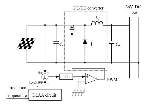
The MPPT efficiency is calculated by the ratio of the energy drawn by the converter within a defined measuring period  $T_M$  to the energy provided by a PV simulator in the MPP. That is:
