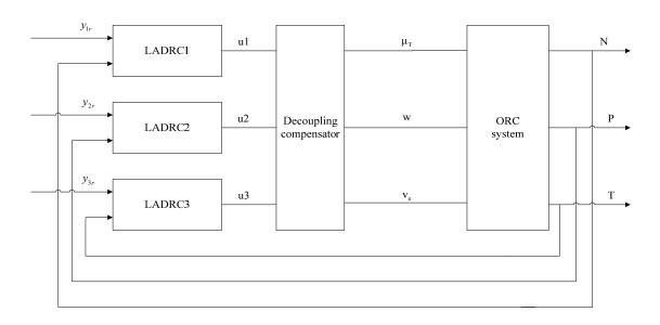
Figure 2. LADRC for the waste heat recovery system.
