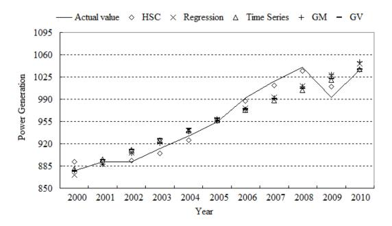
**Figure 4.** Forecasting performance of HS based JPOC model and other four single models for Russian Federation.
