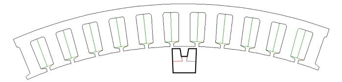
Figure 7. A group of HMPP geometry of the 100-pole, 96-slot machine.
