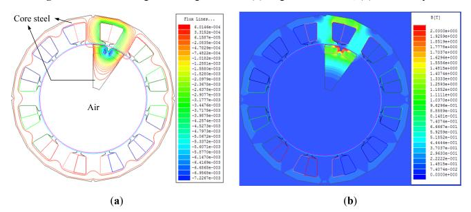
Figure 3. Schematic diagram of magnetic field: (a) magnetic field lines; (b) flux density.
