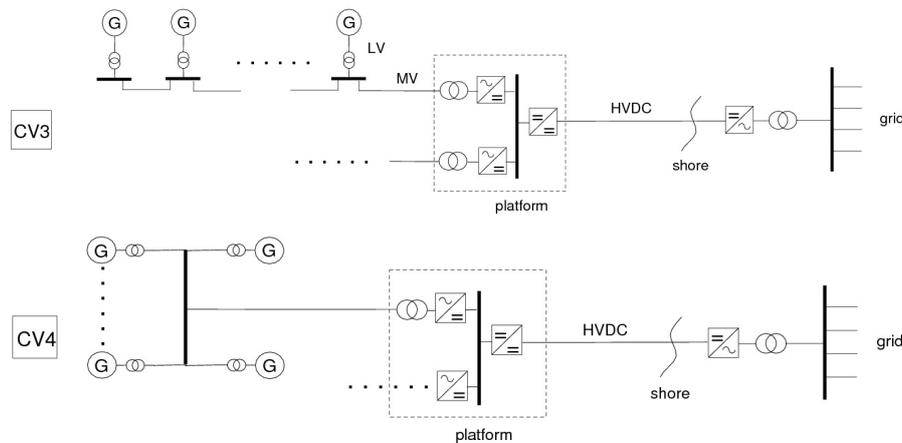
**Figure 8.** Park-coupled variable-speed system with HVDC system.
