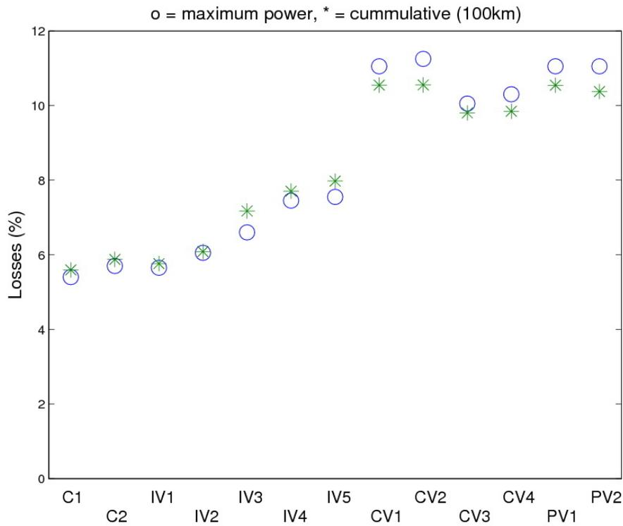
**Figure 11.** PWM converter losses (divided by the rated power): Models compared to typical manufacture data.
