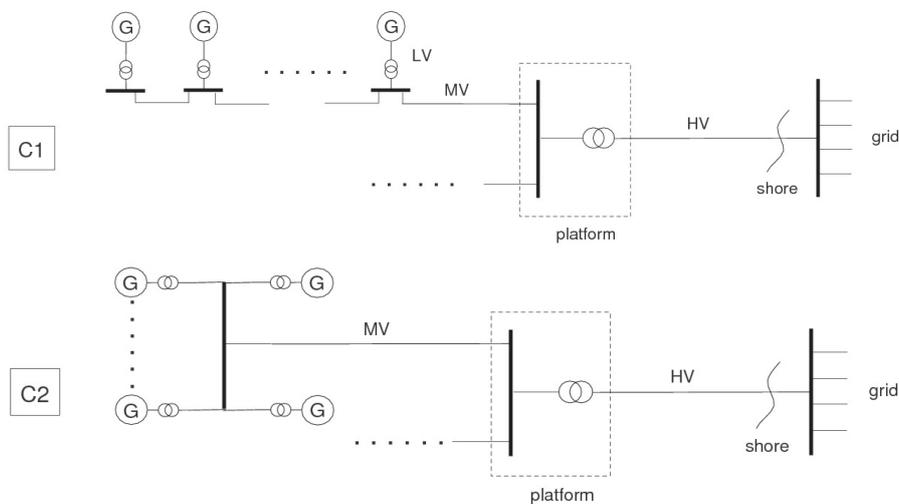
**Figure 4.** Individual variable speed with back-to-back converters.
