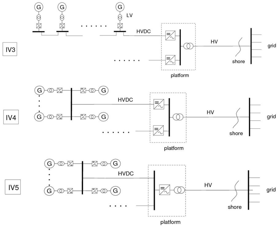
**Figure 6.** Cluster-coupled variable-speed with HVDC system.
