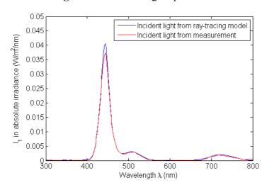
Figure 13. Incident light spectrum.
