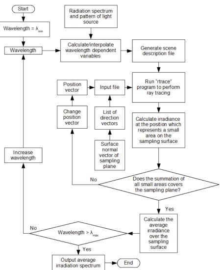
Figure 5. Flow chart of the ray-tracing model.
