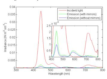
The simulation results for the cases of LSC with mirrors and without any mirror are shown in Figures 17 and Figure 18 respectively, together with the experimental result for comparison. Two peaks were observed in the experimental result.
