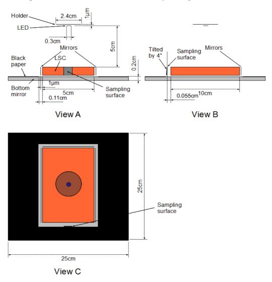
Figure 15. Two-dimensional view of the ray-tracing simulation model.
