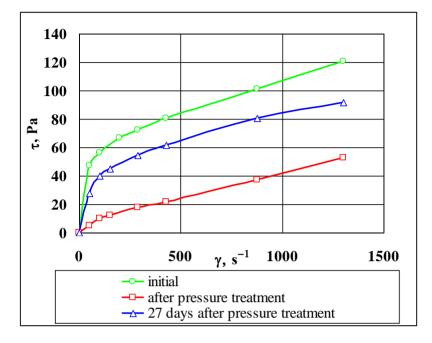
This method of pressure treatment is similar to that mentioned above in the experiment (see Figure 3) and in such a way the pressure treatment of oil in the bottomhole zone can be undertaken. Significant increases of well production have been observed using this procedure on many wells of Shirvan oilfield (Azerbaijan).
