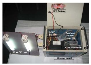
Figure 8. Self-supported DBFC system.
