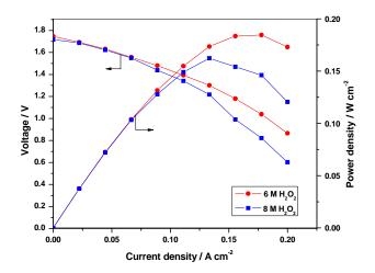
**Figure 3.** Performance data for the DBFC with 6 M and 8 M  $H_2O_2$  in aqueous 1.5 M  $H_2SO_4$  as catholyte and 8 wt. % NaBH<sub>4</sub> as anolyte at a load current-density of 65 mA cm<sup>-2</sup>.
