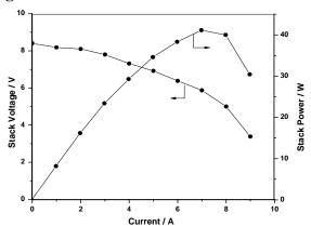
Figure 6. Polarization data for the DBFC stack.
