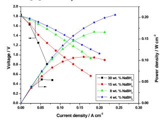
**Figure 5.** Performance data for the DBFC with 4 wt. % and 8 wt. % anolyte and 8 M  $H_2O_2$  as the catholyte at a load current-density of 65 mA cm<sup>-2</sup>.
