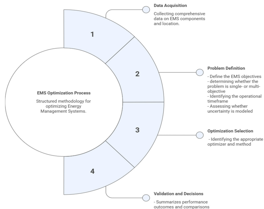
Figure 8. Schematic representation of a standard Energy Management System optimization workflow in microgrids.
