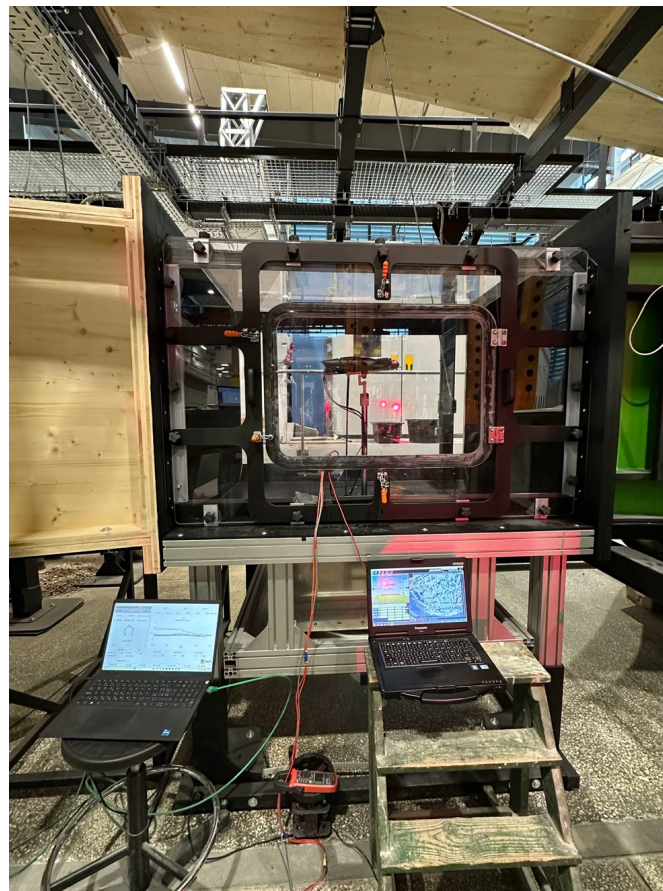
Figure 11. Test stand consisting of a wind tunnel test chamber, two control computers, a laboratory-grade power supply, and a UAV mounted with a strain gauge.
