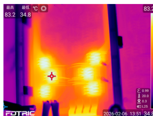
Figure 14. Thermal distribution of M1 under steady-state test. Captions on the upper-left corner shows the highest temperature of 83.2 °C and the lowest temperature of 34.8 °C.
