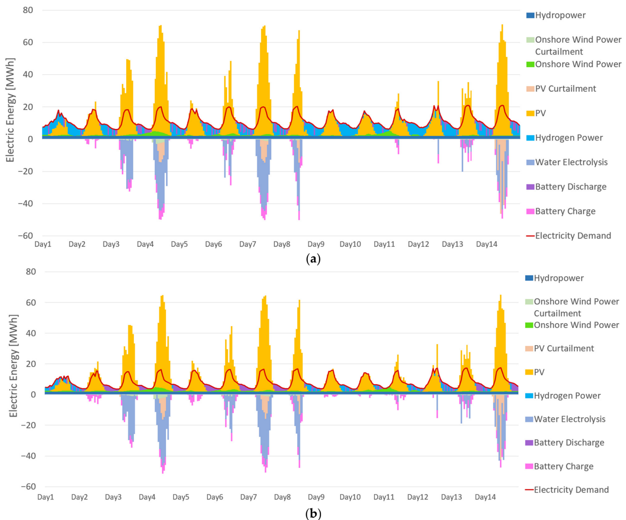
Figure 5. Hourly electricity supply–demand balance: (a) E case; (b) EH case.
