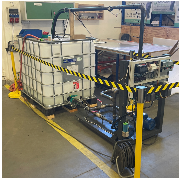
Figure 11. Laboratory test stand for the cooling system controlled by IACMS. Source: Authors' own work.
