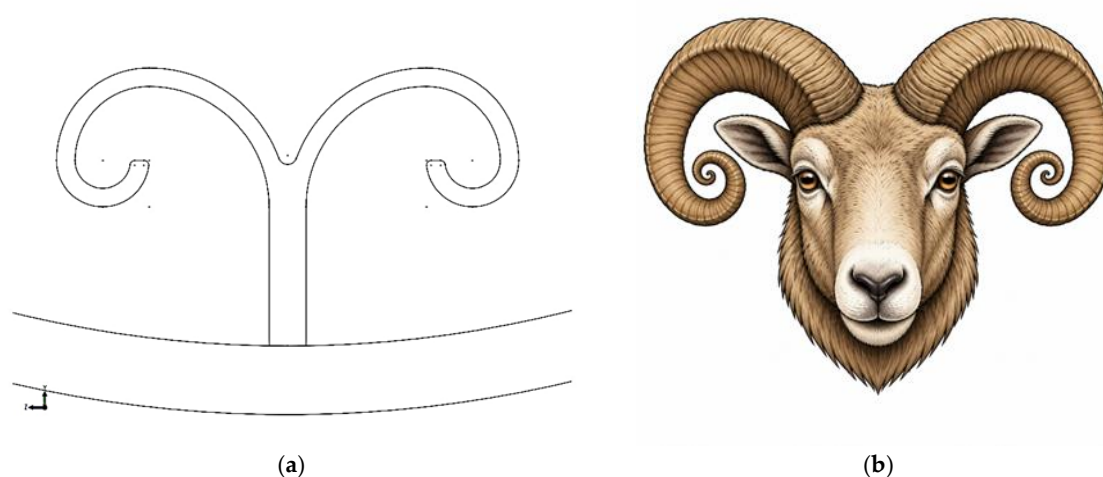
Figure 2. (a) Cross-section of the internal fin, inspired by (b) a ram's horns.
