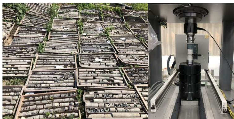
Figure 8. Rock sample coring and uniaxial compressive strength test.
