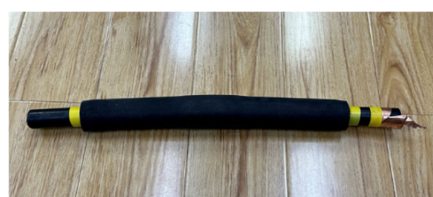
Figure 4. 10 kV Cold-Shrink Cable Joint Sample.
