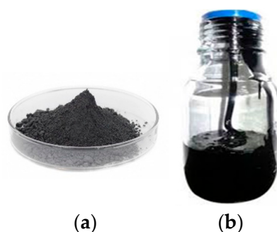
Figure 9. Ex situ catalysts: (a) Mo sulfide ex situ LDPE-stabilized catalyst, (b) Mo sulfide ex situ VR-stabilized catalyst.
