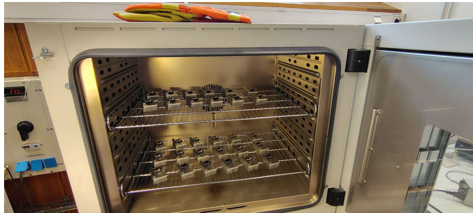
Figure 4. The experiment samples were placed in oven for accelerated lifetime test.
