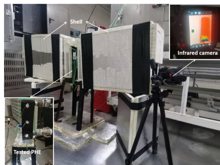
Figure 2. Infrared temperature measurement devices.
